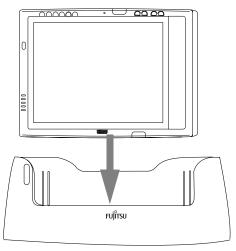
Figure 3. Installing the Tablet PC in the Cradle
